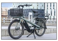
Class 1—Pedal assisted only; motor cuts out at 20 mph. If operating on a sidewalk, the motor cannot be engaged. On the road, rider must obey all traffic laws. Front white light and back red light and reflectors required.
