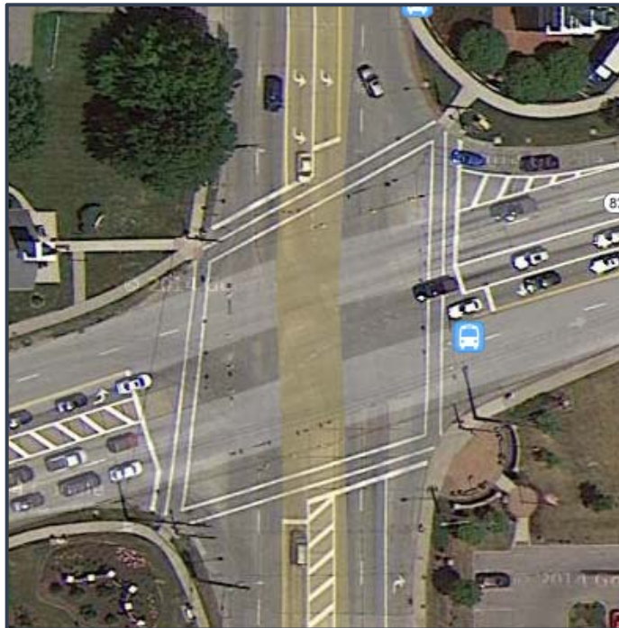
Figure 5 | Pearl and Royalton Roads Intersection with and without pedestrian refuges and porkchop island recommendations
