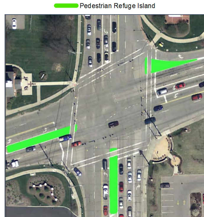
Figure 5 | Pearl and Royalton Roads Intersection with and without pedestrian refuges and porkchop island recommendations
