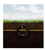
Before attempting to clear a blocked sewer line, call 811 so that utility lines can be marked. It's the best way to ensure the sewer line is free of cross-bores and to avoid a potentially unsafe situation. For more information on cross bores, visit <a href="columbiagasohio.com/safety/natural-gas-safety/sewer-line-safety">columbiagasohio.com/safety/natural-gas-safety/sewer-line-safety</a>. If you believe you have a cross bore, call 1-800-344-4077.
