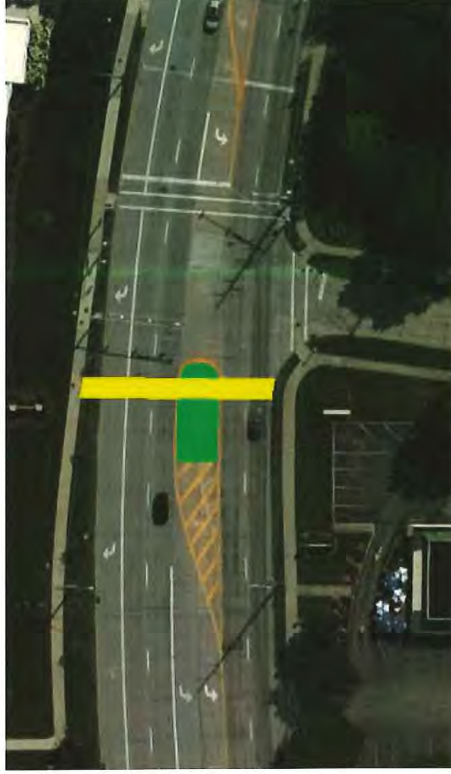
Figure 10 | Pearlview Drive and Royalton Road intersection with proposed crosswalk and pedestrian refuge island
